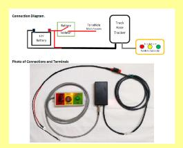
A minimum of 100mm of Track Race Power Supply Cable and Console cable should be left at the unit mounting location for connection to the unit.
